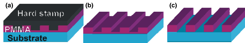
Figure 1.6. Schematic diagram of the nanoimprint lithography process. (a) Imprinting with a stamp creates a thickness contrast into a deformable polymer layer. (b) Removal of the stamp retains the pattern. (c) Pattern transfer into the polymer using anisotropic etching to remove the residual polymer layer in the compressed areas.
